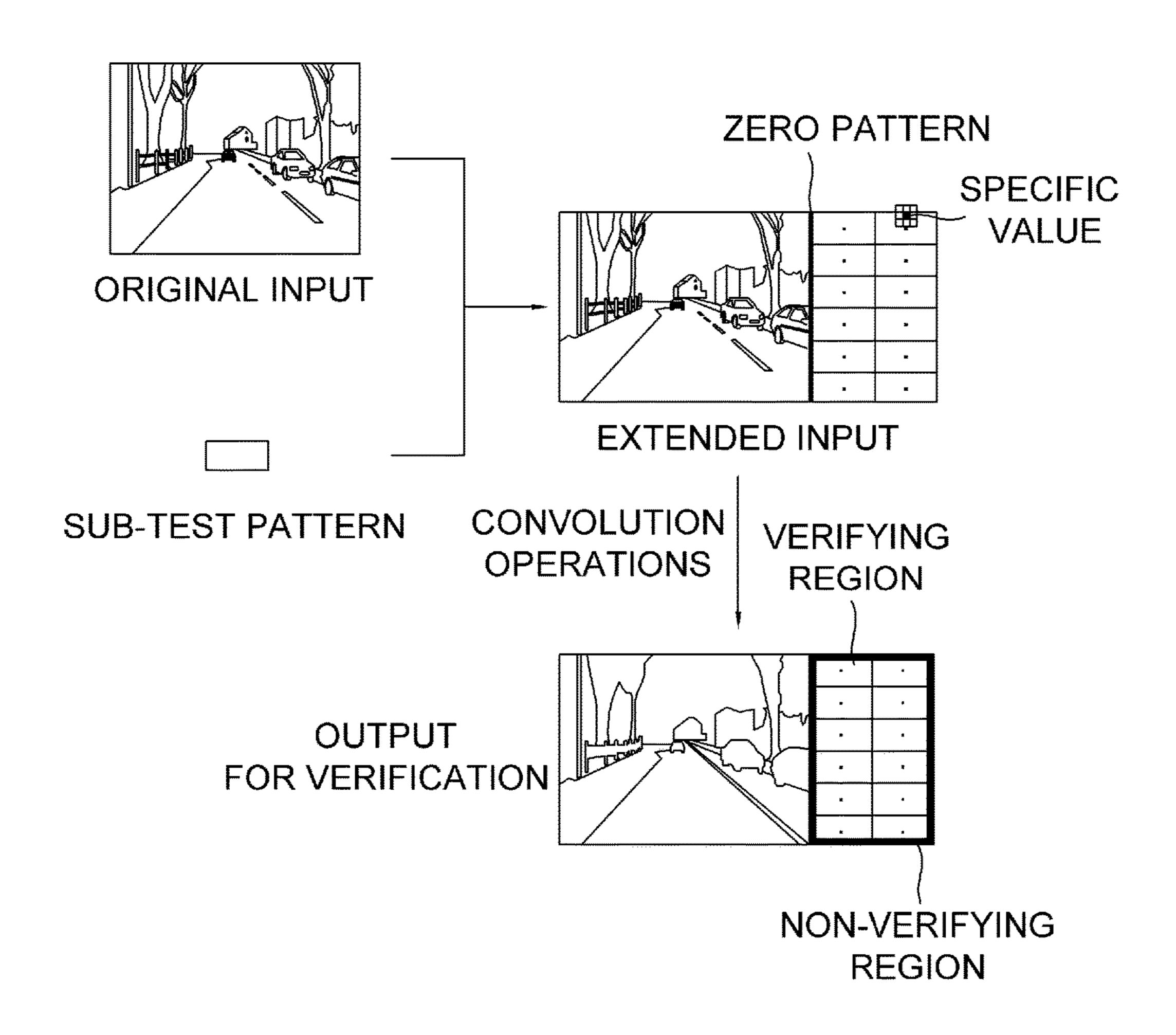
METHOD AND DEVICE FOR VERIFYING INTEGRITY OF PARAMETERS OF CNN BY USING TEST PATTERN TO ENHANCE FAULT TOLERANCE AND FLUCTUATION ROBUSTNESS IN EXTREME SITUATIONS FOR FUNCTIONAL SAFETY
