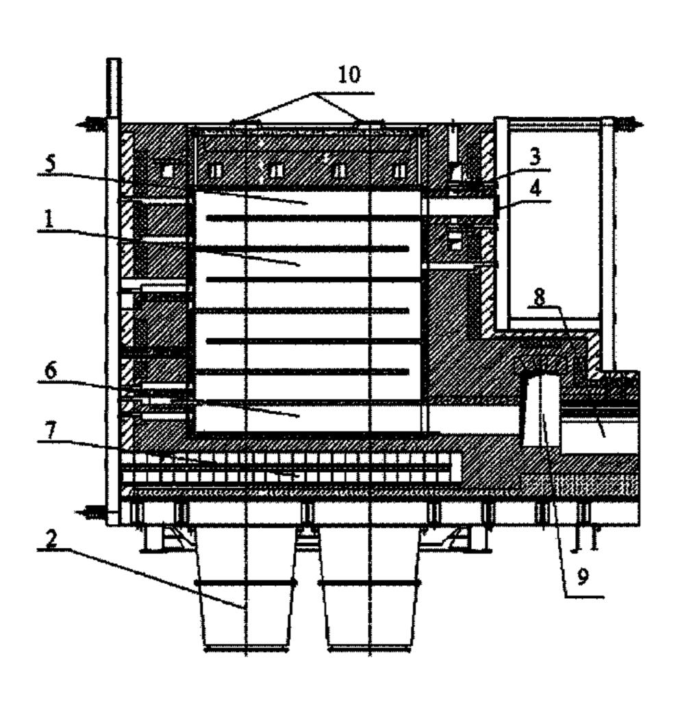
is provided with a first flame path layer flashboard An eighth flame path layer may be in communication with a communication flue. Flue gas may be discharged out of the furnace body through a main flue. A furnace bottom cooling channel may be provided below the eighth flame path layer.
