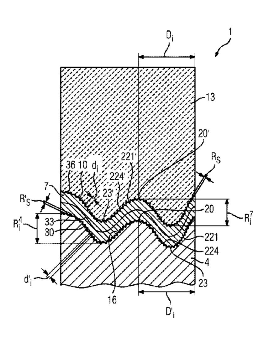
positioned on an interface of the layers located above, and the adhesion of the layers to one another is thereby improved.
