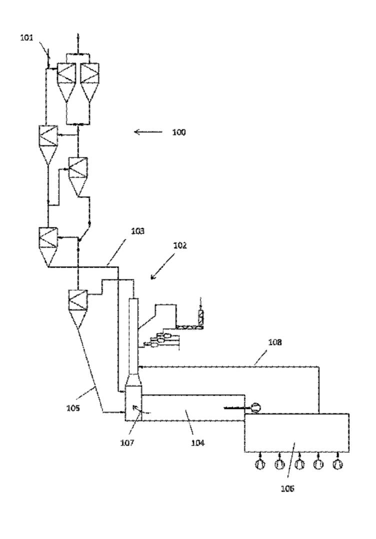
fuel is dried and/or at least partially de-gassed and/or at least partially reacted and subsequently transferred into the riser tube.
