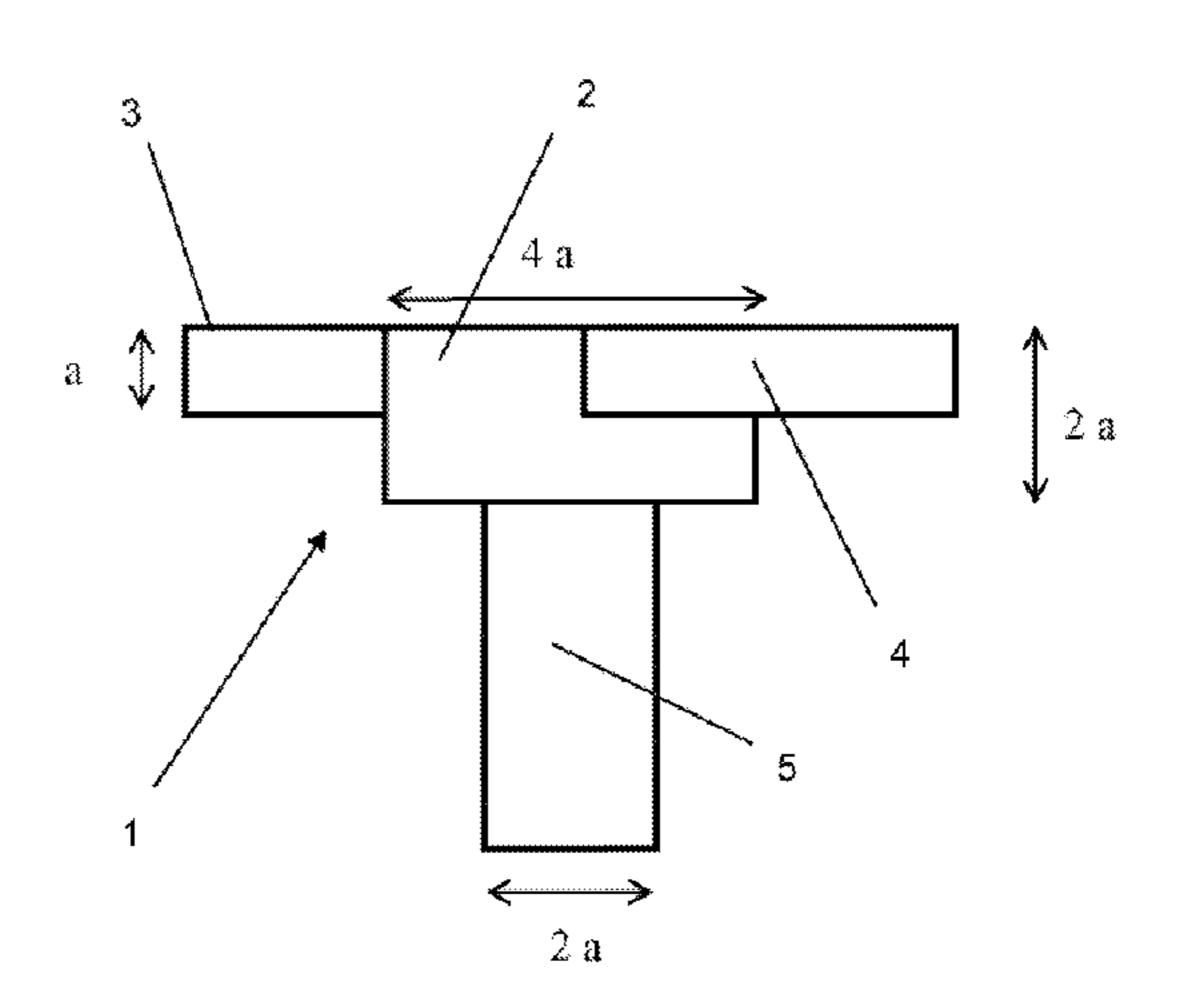
a basic compound with a residence time of the reaction medium in the mixing zone of the reactor of at most 100 milliseconds; the precipitate is heated then brought into contact with a surfactant before being calcined.
