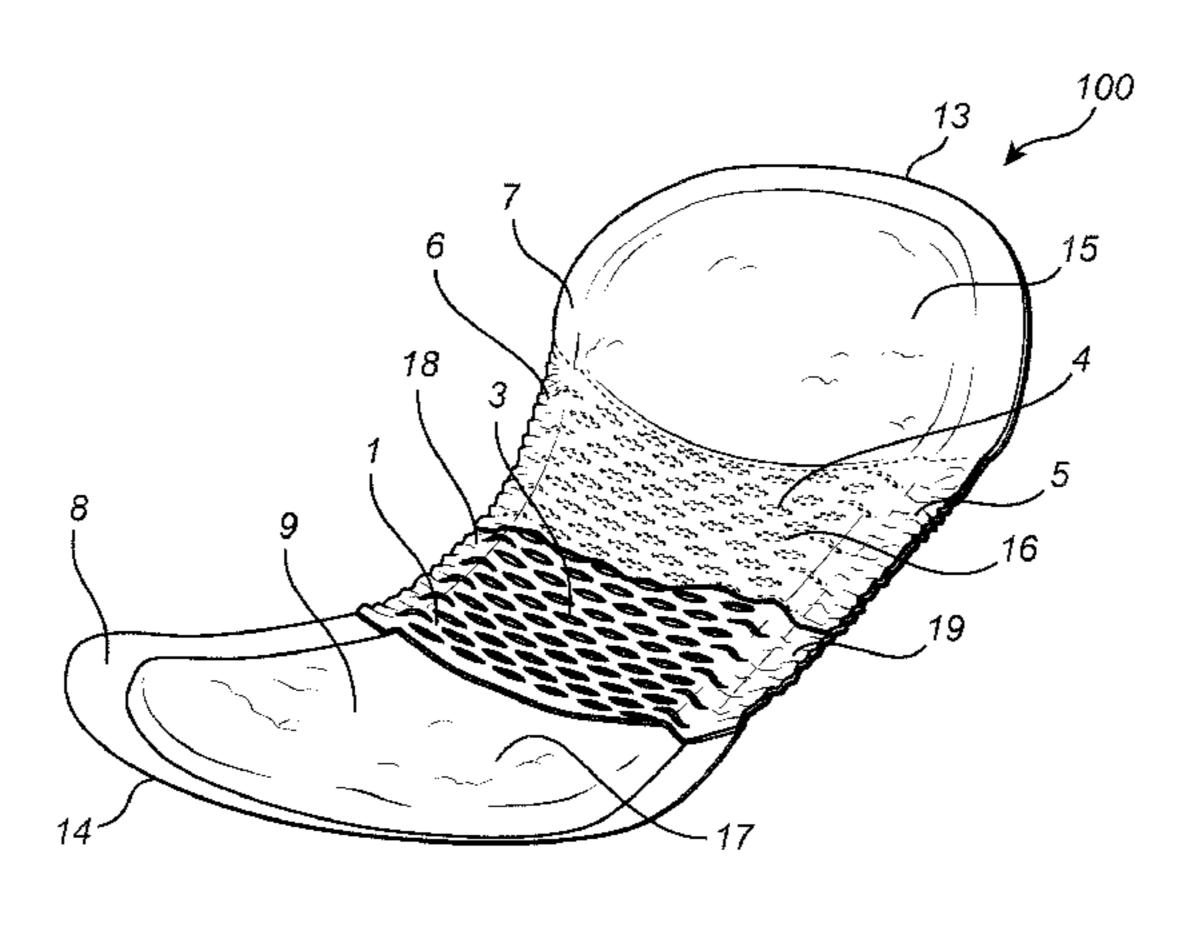
has in its transversal direction of the absorbent product a central region and two edge regions. The openings are located in the central region so that the central region of the material with the plurality of openings has a lesser degree of elasticity than the edge regions.
