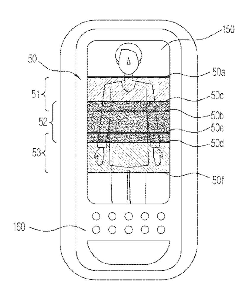
ler to control the X-ray generator to perform segmentation imaging with respect to the designated region.
