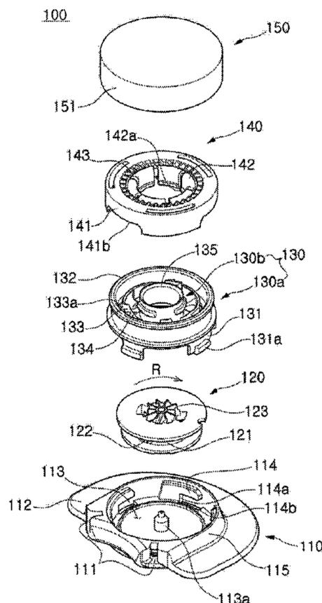
gear protruding from an inner circumference thereof; and a cover part coupled to an upper portion of the vertically moving gear part.
