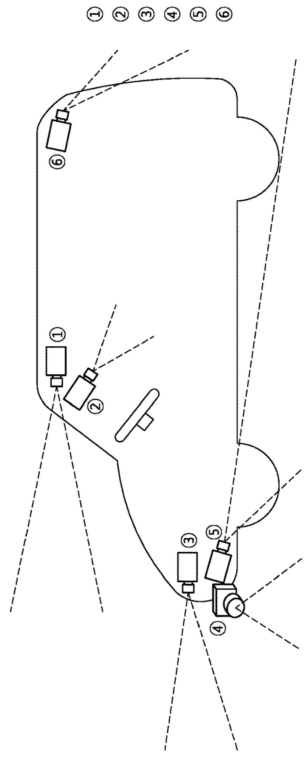
① Headway Sensing Camera② Interior Sensing Camera
