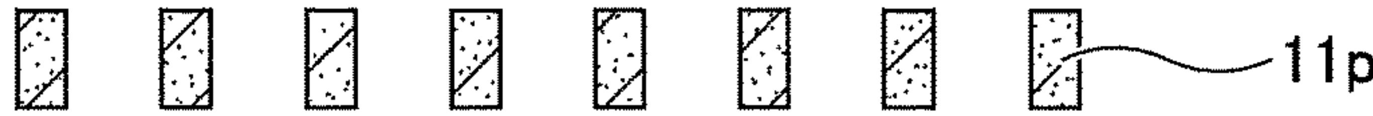
FIG.6E REMOVE SILICON OXIDE FILM
