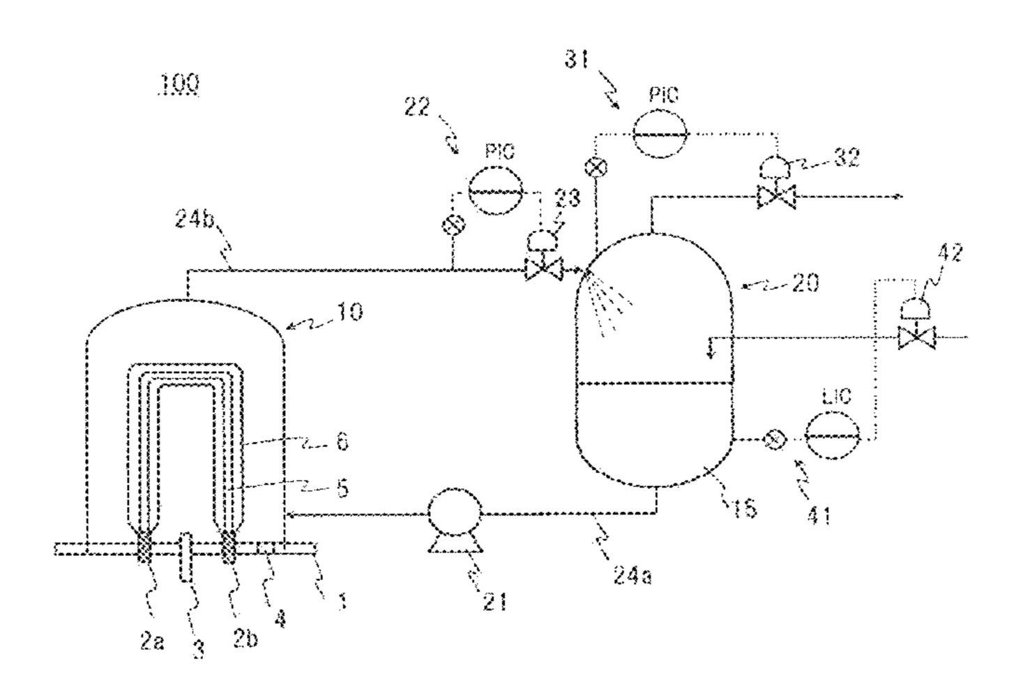
reactor inner wall is kept at a temperature of not more than 370° C. Additionally, the pressure of the hot water 15 to be recovered is reduced by a pressure control section provided in a coolant tank 20 to generate steam. Thereby, a part of the hot water is taken out as steam to the outside, and reused as a heating source for another application.
