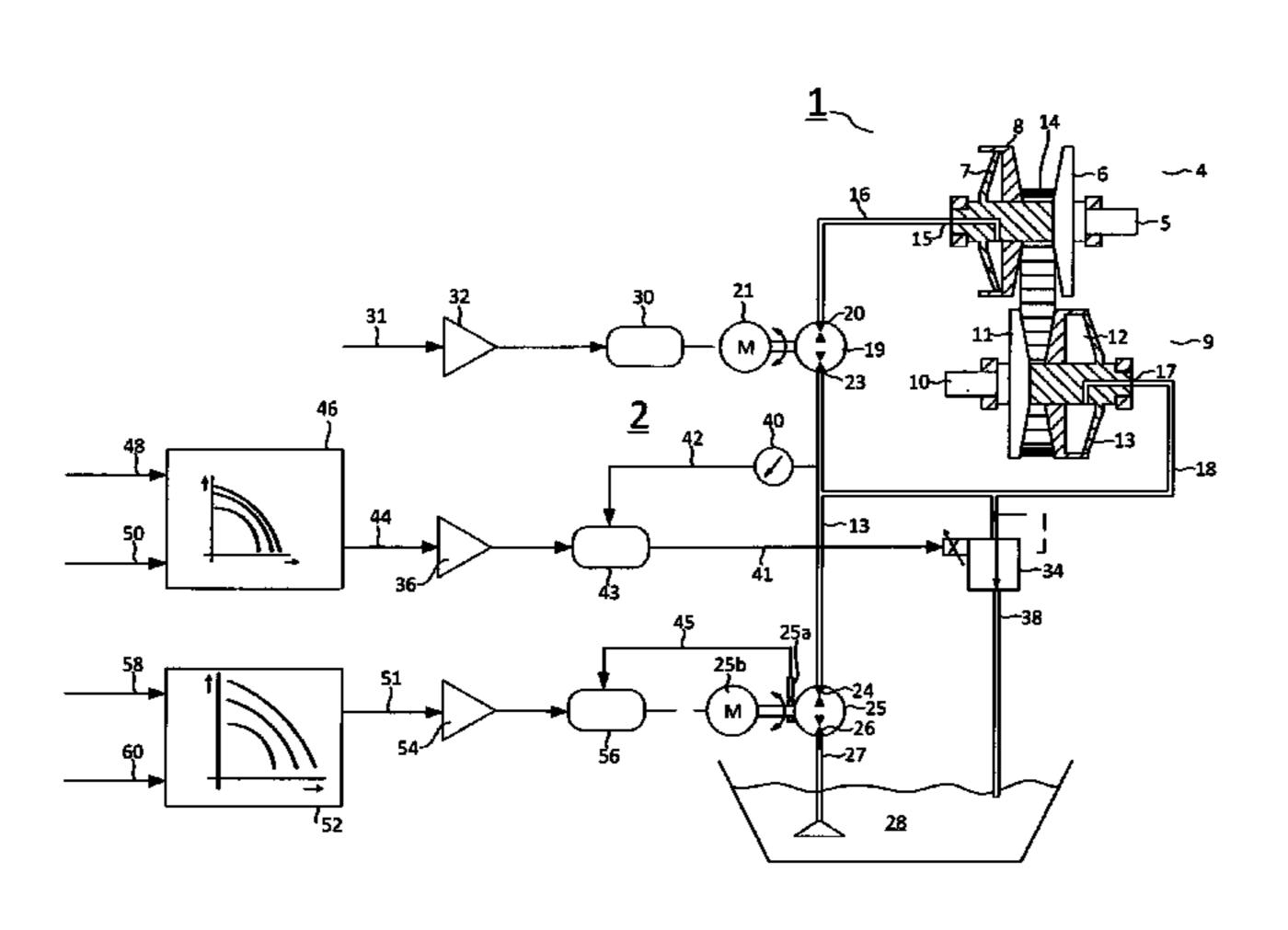
set point is determined by a second control signal as a function of the set transmission ratio on one hand and the value of the actual torque transmitted through the transmission on the other hand, in such a way that de value of the resulting hydraulic pressure increases as the transmission ratio increases on one hand, and as the torque transmitted through the transmission increases on the other hand.
