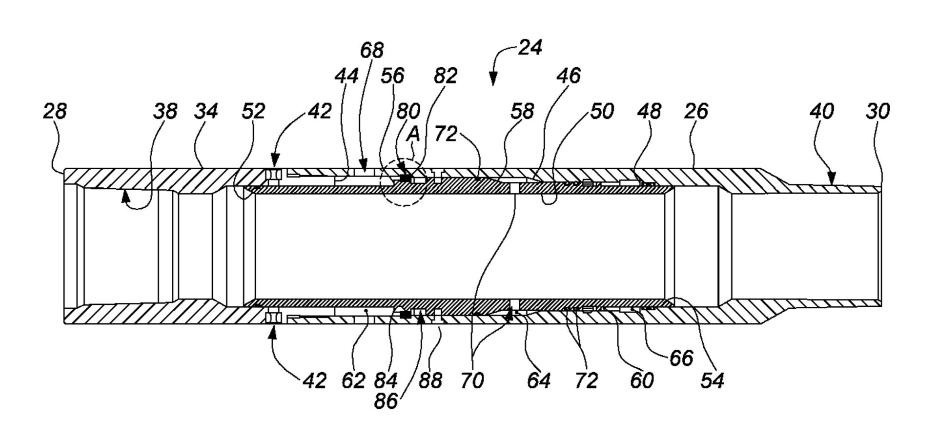
chamber to draw the sleeve towards a second end of the outer mandrel thereby uncovering the valve openings.
