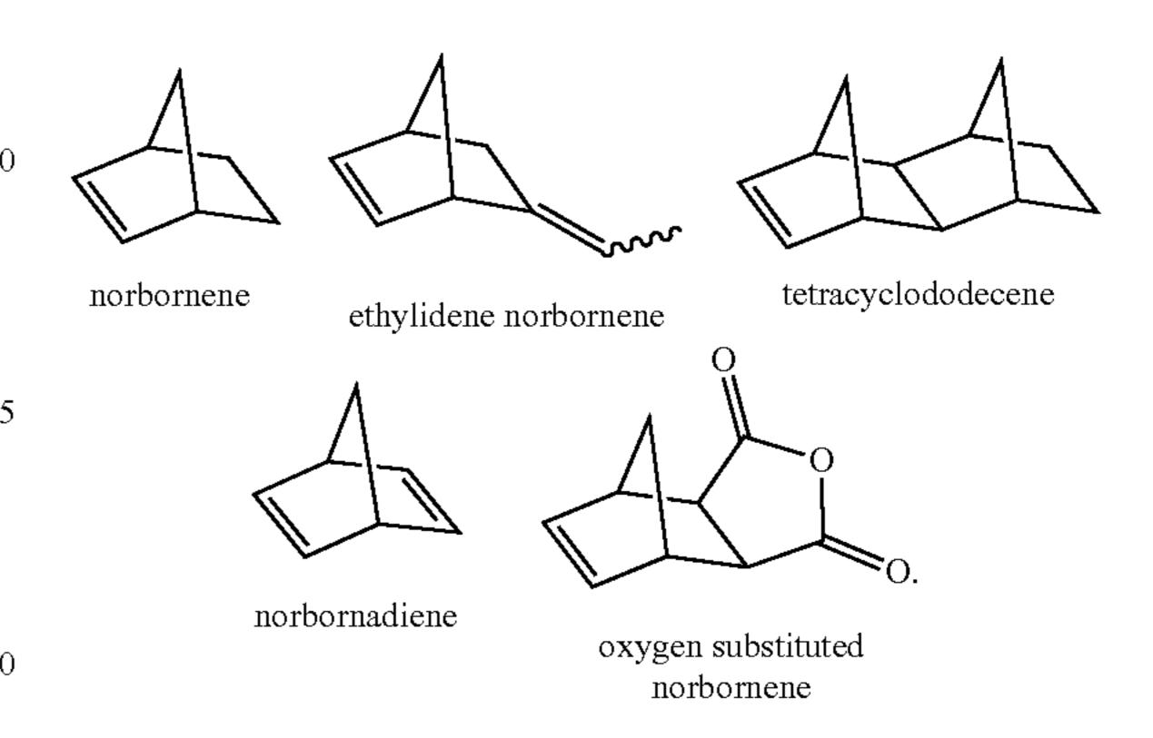
The foregoing Diels-Alder reaction products are useful for producing polymers and copolymers of cyclic olefins copolymerized with olefins such as ethylene. The resulting cyclic olefin copolymer and cyclic olefin polymer products are useful in a variety of applications, e.g., packaging film.
