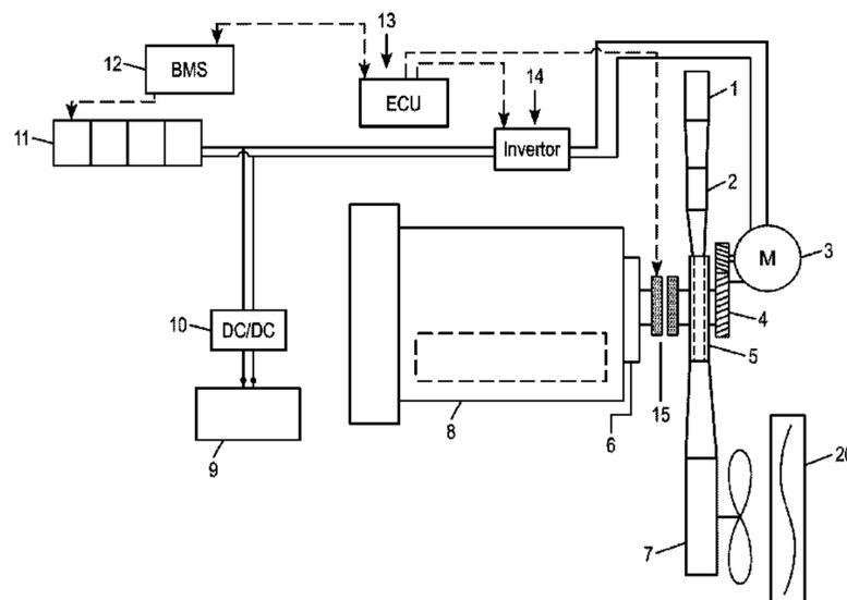
damper to drive the engine accessories using energy returned from the energy store, independent of the engine crankshaft.
