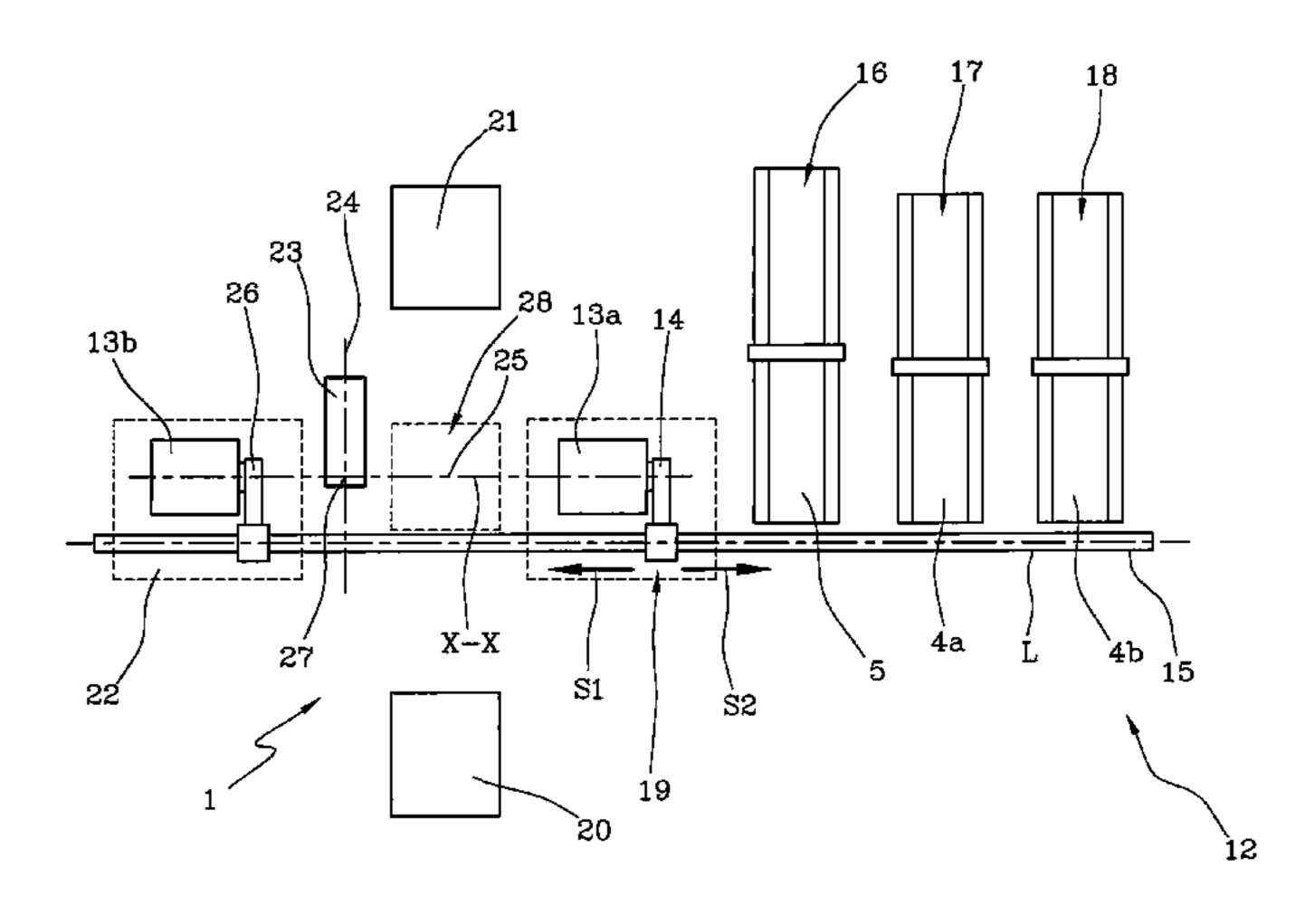
assembling with a crown structure to a second transfer location. At an operating moment in which the first transfer location is occupied by a forming drum coming from the intermediate forming line or intended for the intermediate forming line, from one to n locations selected from the n completion locations and the second transfer location are occupied by respective forming drums.
