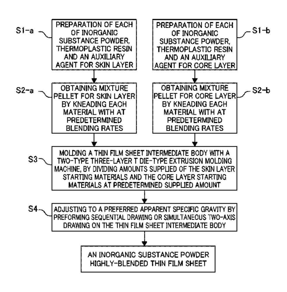
and molding a sheet, and a step for adjusting the apparent gravity as desired by stretching under predetermined conditions.
