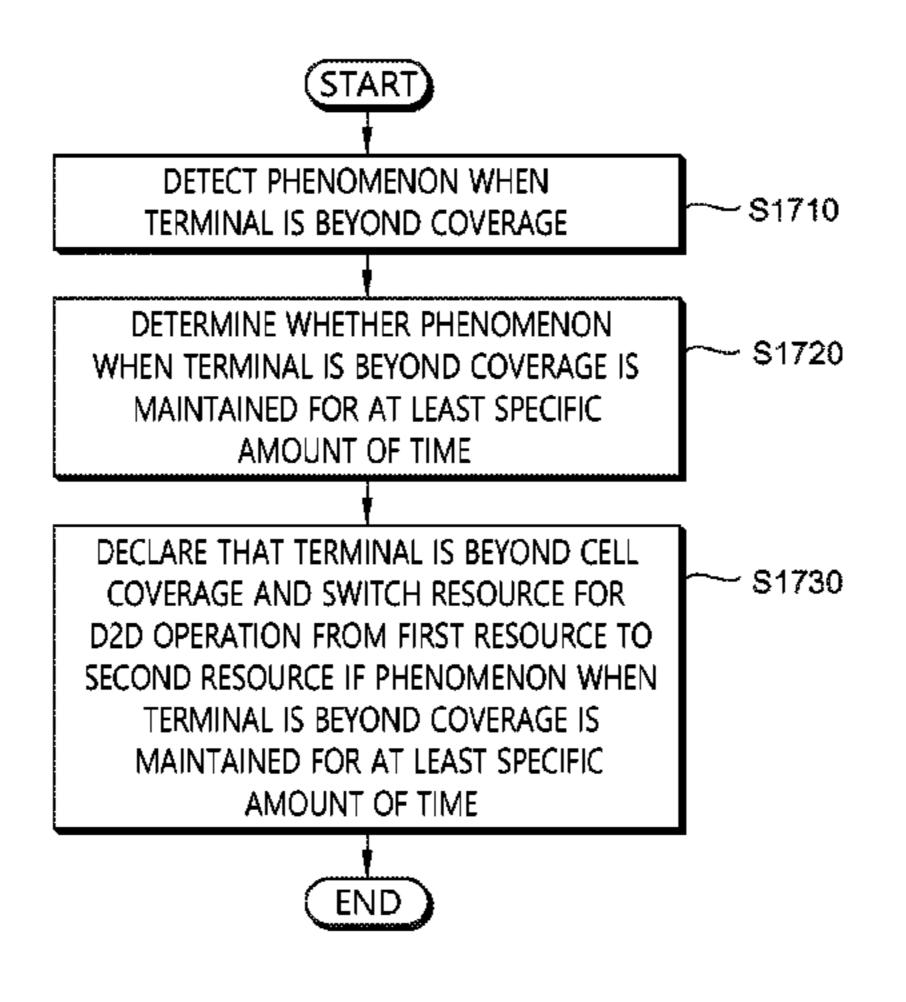
when the successful detection of the specific signal is not maintained for at least the specific amount of time.
