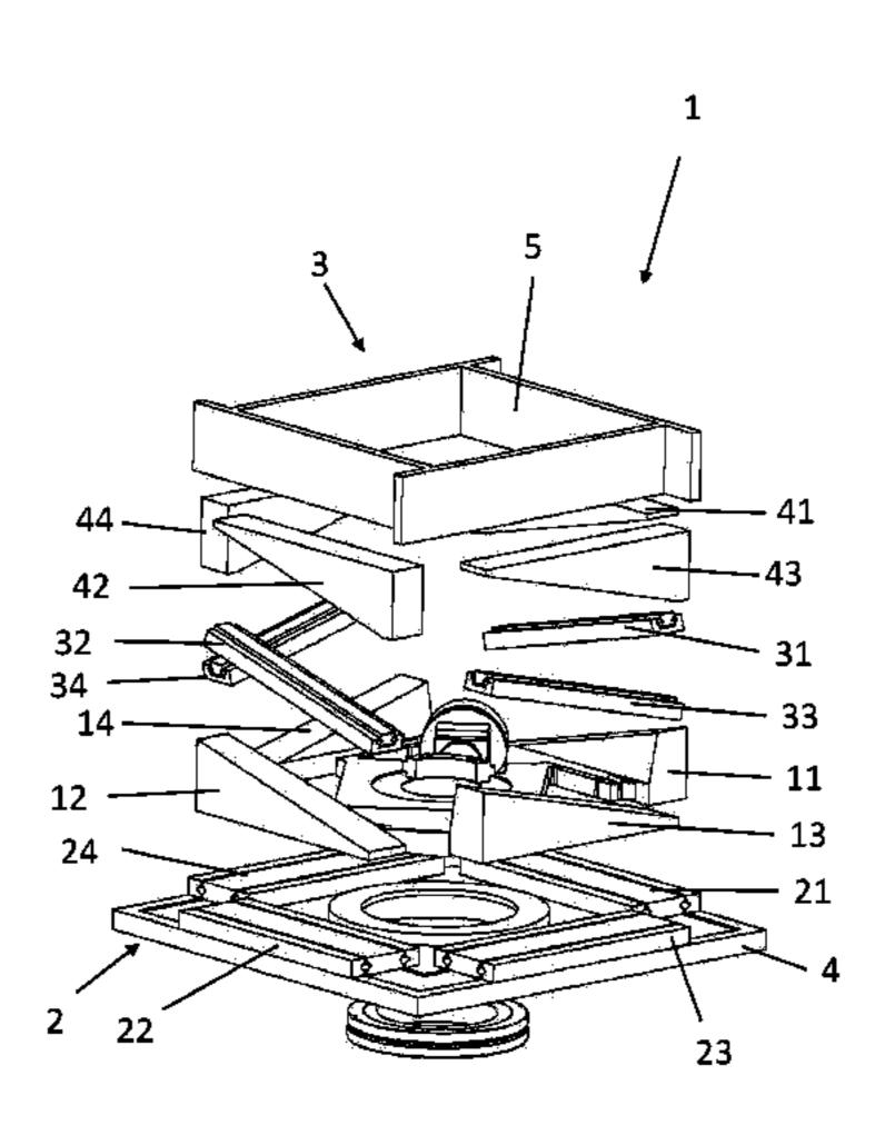
synchronous displacement of the first, second, third and fourth slide element relative to the base element brings about a displacement of the carrier element relative to the base element exclusively along the z-axis.
