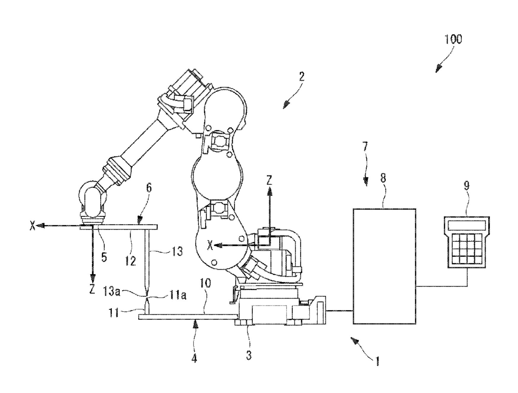
includes a positional offset calculating unit configured to calculate an offset amount of a zero point of each axis of the robot from a true zero point of the axis based on a plurality of sets of the positional data stored in the axial position recording unit.
