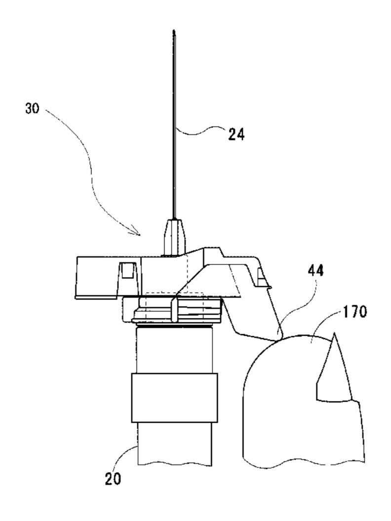
injection needle. The force receiving portion has an easy sliding portion, which is disposed in an area adjacent to an injection needle, and slides more easily along the injection needle than a case where an edge slides along the injection needle.
