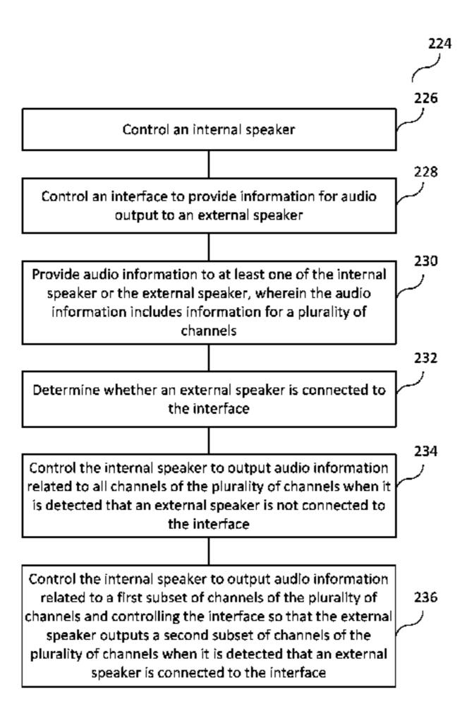
channels and to control the interface so that the external speaker outputs a second subset of channels of the plurality of channels when the determination circuit detects that an external speaker is connected to the interface. According to various embodiments the audio may be processed by a custom HRTF and or DSP in order to improve audio fidelity and user experience.
