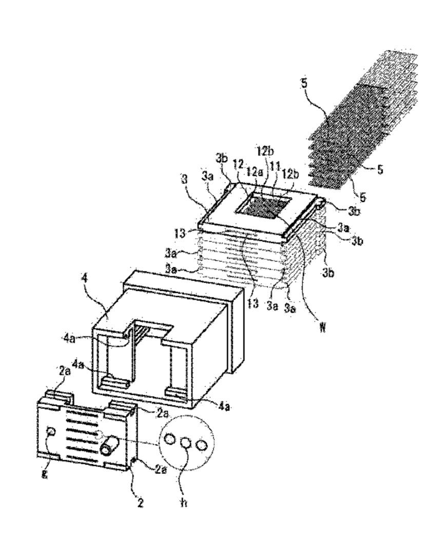
connected at the time of connecting the connectors, and furthermore, positioning accuracy between the respective fibers 5 can be improved when the connector is used as a multi-fiber optical connector 1.
