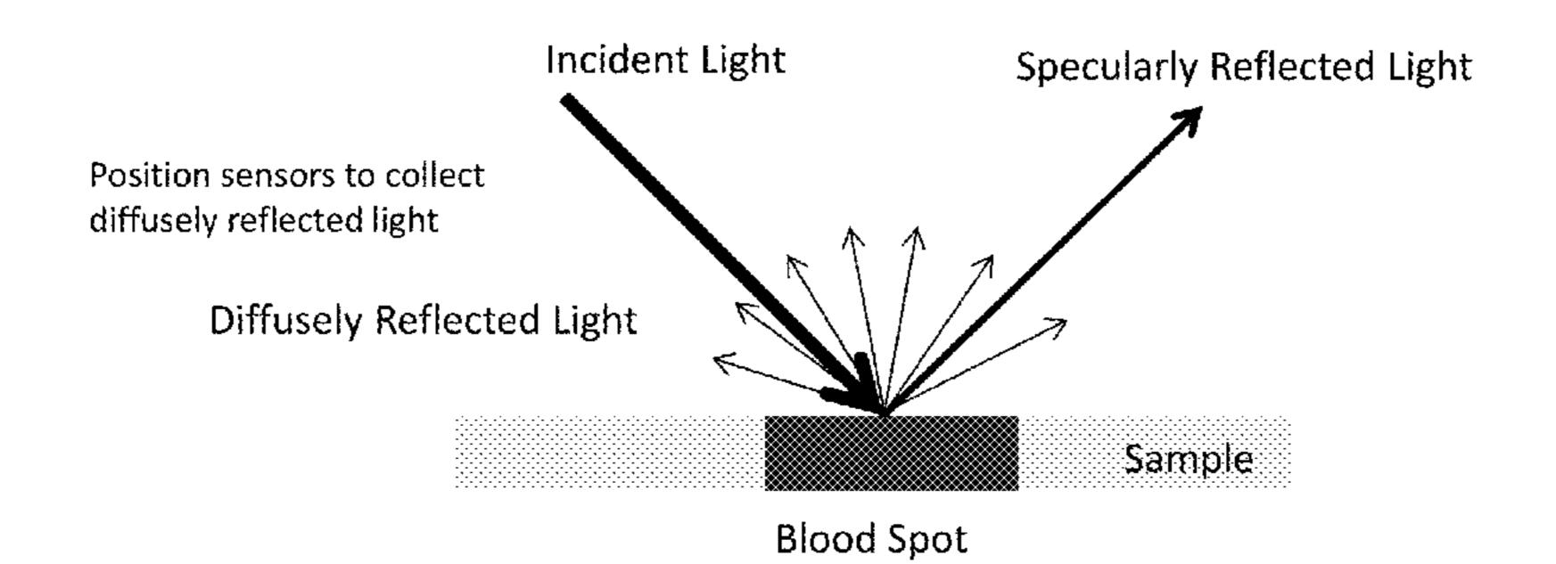
Do not position sensors to collect light transmitted all the way through the sample
