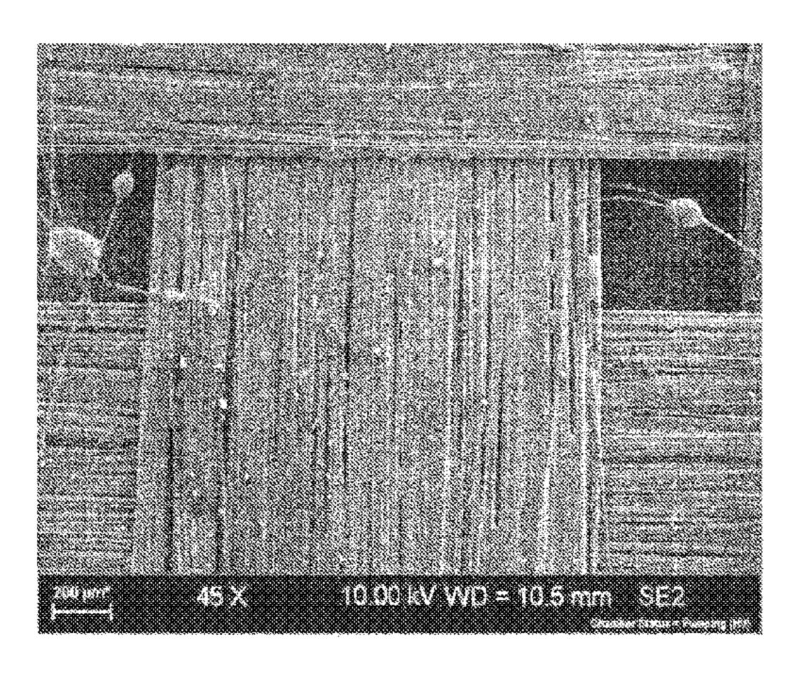
wherein the reinforcing fiber substrate has void space that is opened on an outer surface thereof and the resin is in a semi-impregnated state.
