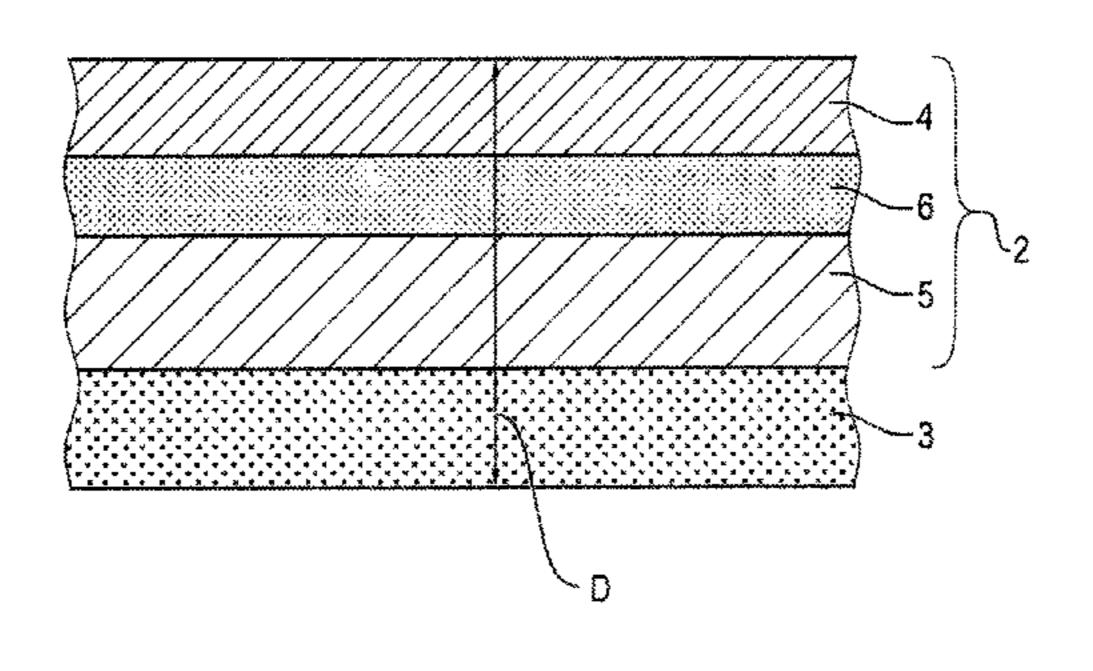
312, and enabling easy processing with a minimal thickness, the first and second textile layers (4) each have a basis weight ranging from 80 to 300 g/m<sup>2</sup>, the adhesive connection layer (6) having a basis weight ranging from 50 to 300 g/m<sup>2</sup> and a laminate adhesive force, by DIN EN 1939, between the textile layers greater than 10 N/cm.
