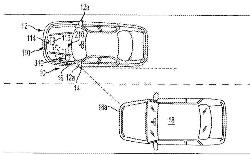
consisting of (i) captured image data and (ii) captured radar data, detects another vehicle that is present exterior of the equipped vehicle.
