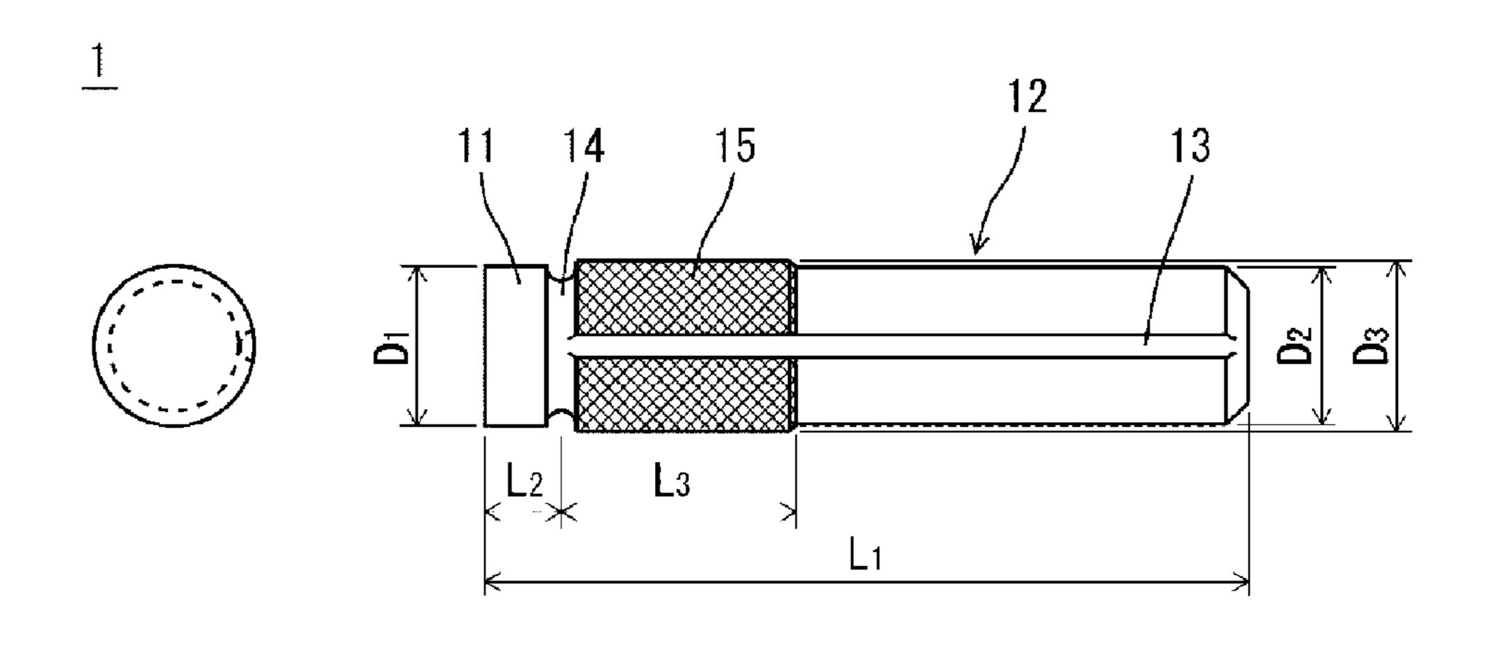
surface of the prepared hole. A vent piece has a saw cut extending in the axial direction formed on the side surface of the cylinder.
