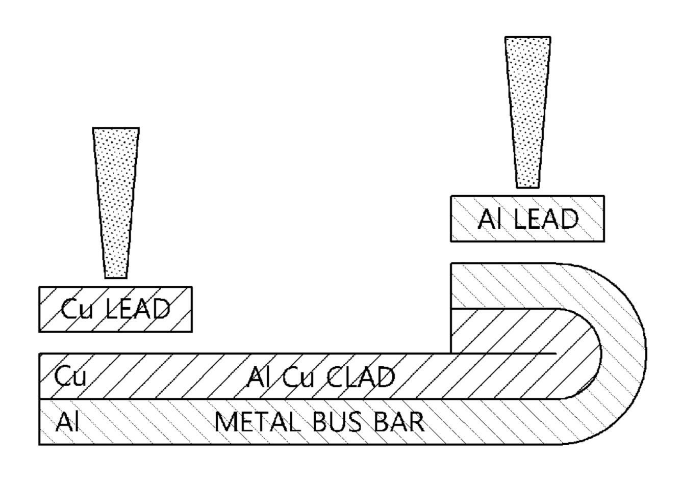
solving cracking or corrosion problems of a conventional welding process and also welding an over-lay clad metal with leads, thereby generating economic benefits and increasing the convenience of the welding process.
