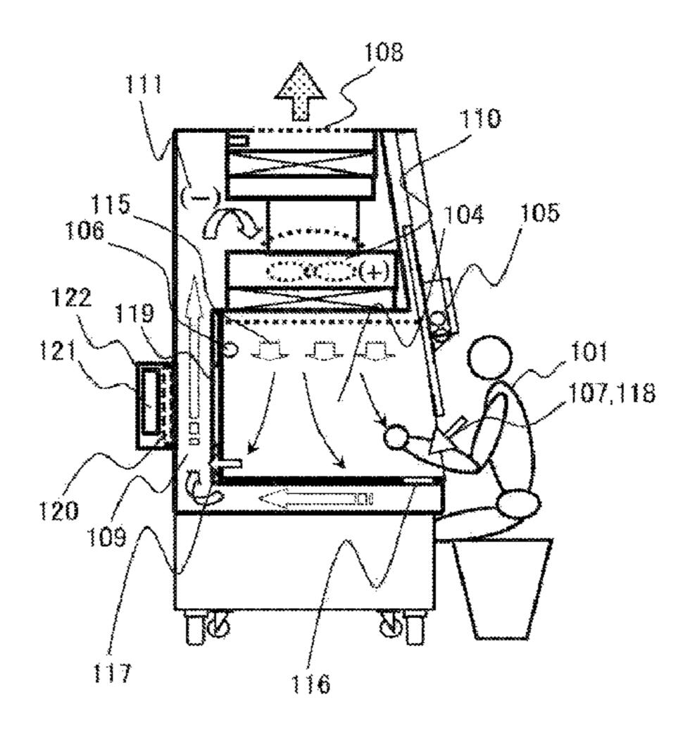
wall or a side wall of the body of the safety cabinet separated from the back wall or the side wall of the work space by a circulation flow path, which allow the operator to see through both walls, and the display device is placed on an outer side portion of the transparent window provided at the portion of the rear wall or the side wall of the body of the safety cabinet.
