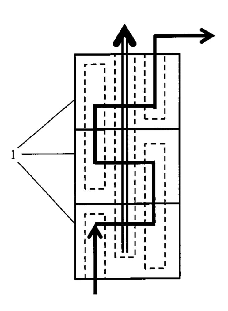
ments to serialize the flow path of the feed and retentate without requiring diverter plates.
