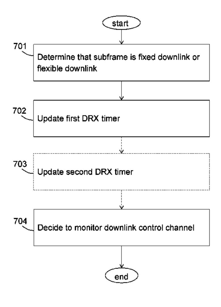
figured to operate as a downlink subframe, the UE decides, to monitor the downlink control channel in the subframe.
