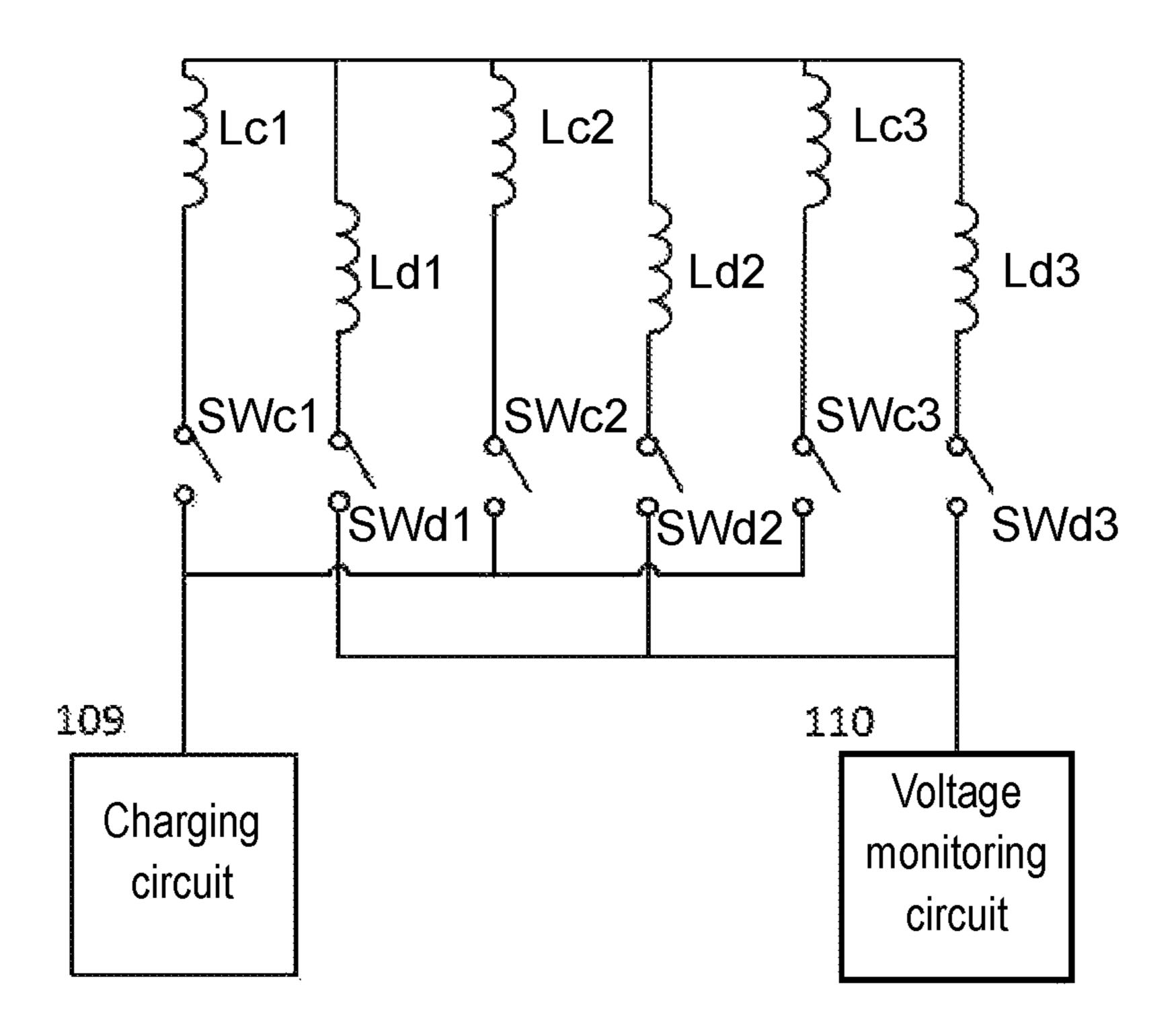
F/G. 6 START S101 Detect initial position of object to be charged S103 Start charging by charging coil Lc\_2 closest to initial position S105 Measure coil-end voltages V1, V2, and V3 of position detection coils S107 V1/V2 or V3/V2 exceeds threshold? No YES S109 Switch to adjacent charging coil **END**
