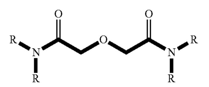
wherein R is an alkyl selected from the group consisting of normal or branched derivatives of DGA and combinations thereof. The resin works by solvating cations with an inorganic counter-ion in the solubilized titanium liquor.
