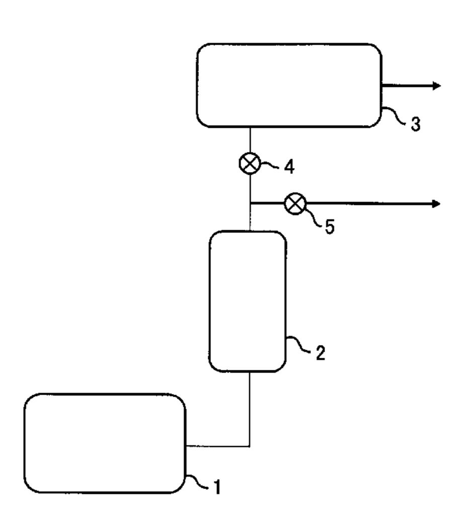
water vapor not adsorbed by the adsorbent. The method also includes a desorption step of maintaining vapor pressure around the predetermined adsorbent which has adsorbed the water vapor in a range in which light water is desorbed and heavy water or semi-heavy water is not easily desorbed, and recovering the water vapor desorbed from the adsorbent.
