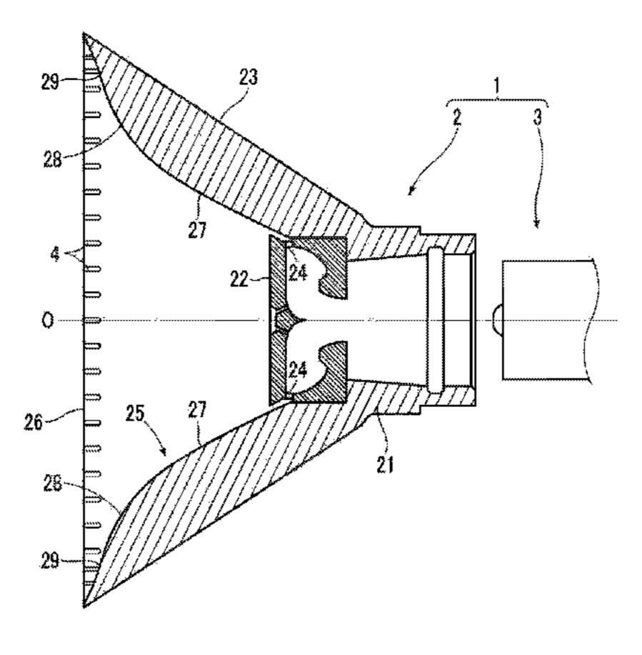
large diameter side having a curved surface with a concave shape towards the axial line (O) with grooves (4) on the outer edge (26).
