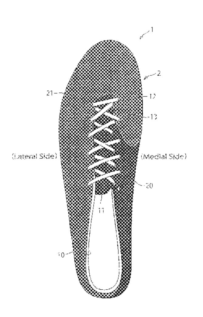
22, respective end portions 20E, 21E of the expandable part 20 and the non-expandable part 21 are sewn together such that a seam does not appear on the boundary surface. The shoe may further include an outsole having at least one groove in a particular triangular region on a bottom surface of the outsole.
