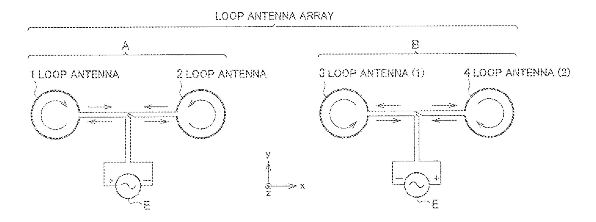
source, a counterclockwise current flows through one loop antenna while a clockwise current flows through the other loop antenna.
