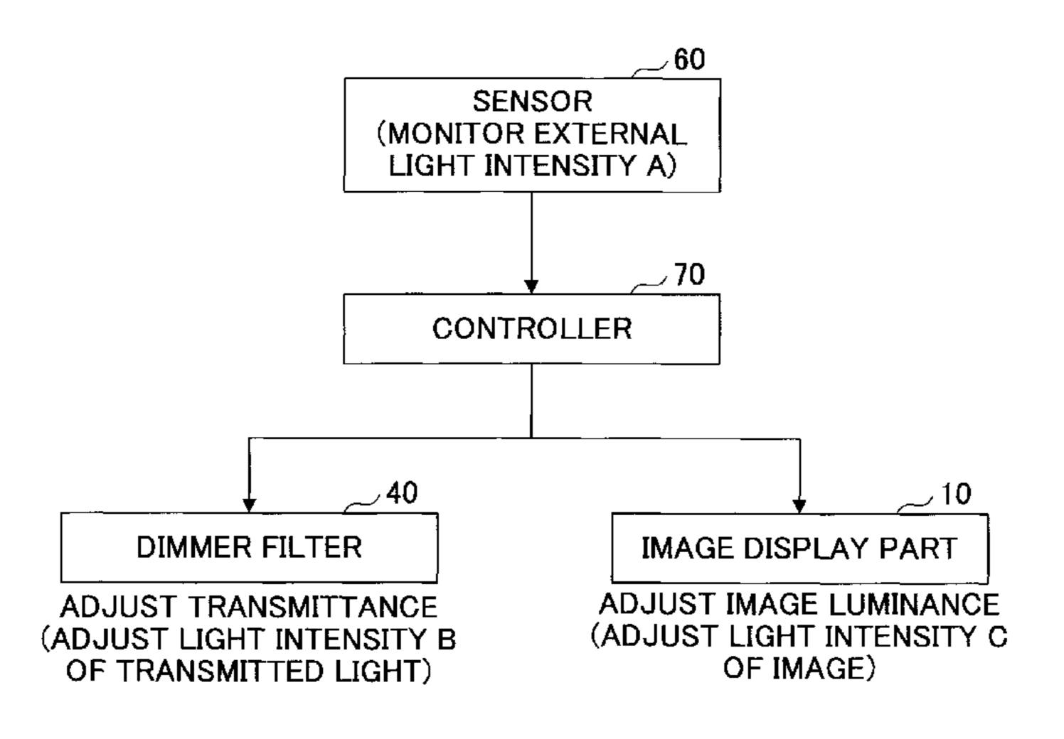
figured to adjust the transmittance of the dimmer filter (40) and the light intensity (C) of a light source of the image display part (10) based on the light intensity (A) of the external light obtained by the light intensity detector (60).
