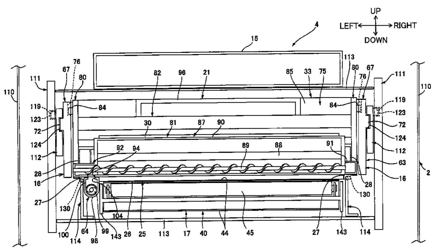
waste toner collected from drums and conveys collectively the aggregated waste toner to the waste toner cartridge.
