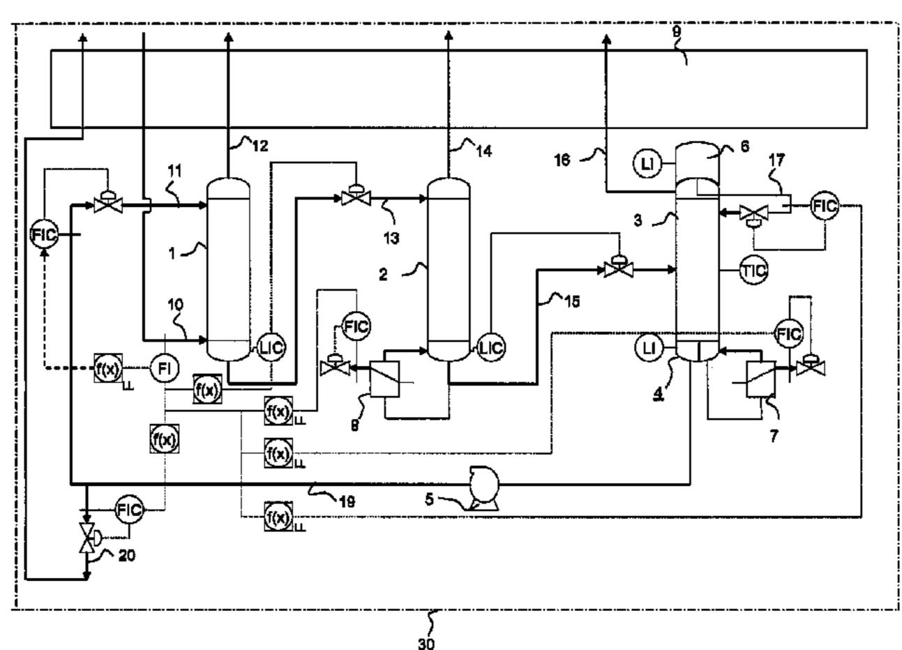
separated in a separation column to produce a gas enriched in carbon monoxide and a liquid methane flow at least part of which forms a purge stream, the purge stream being varied to take account of load variations.
