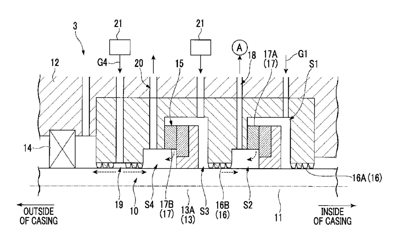
by mixing the process gas, which is compressed by the compressor, and the inert gas, which is supplied to a seal portion of the compressor.
