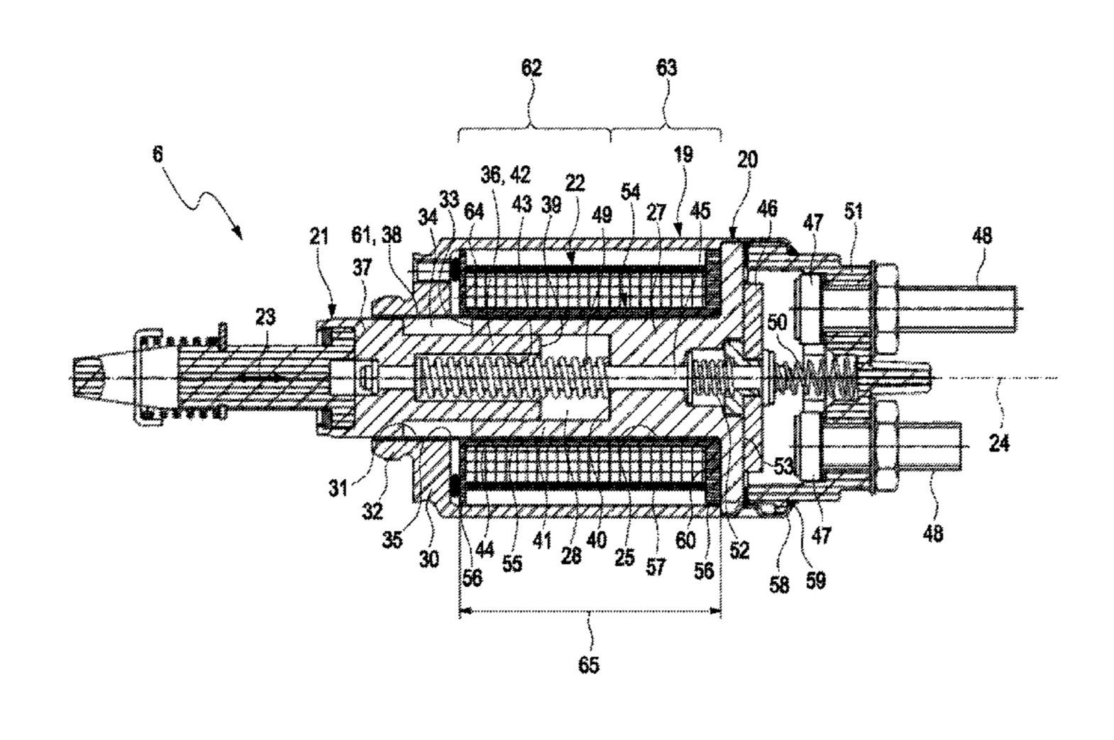
coil arrangement arranged in the solenoid housing surrounding a cylindrical coil interior in a circumferential direction. The plunger stop may include a cylindrical section projecting axially into the coil interior. The cylindrical section may have a face end facing towards the face side wall.
