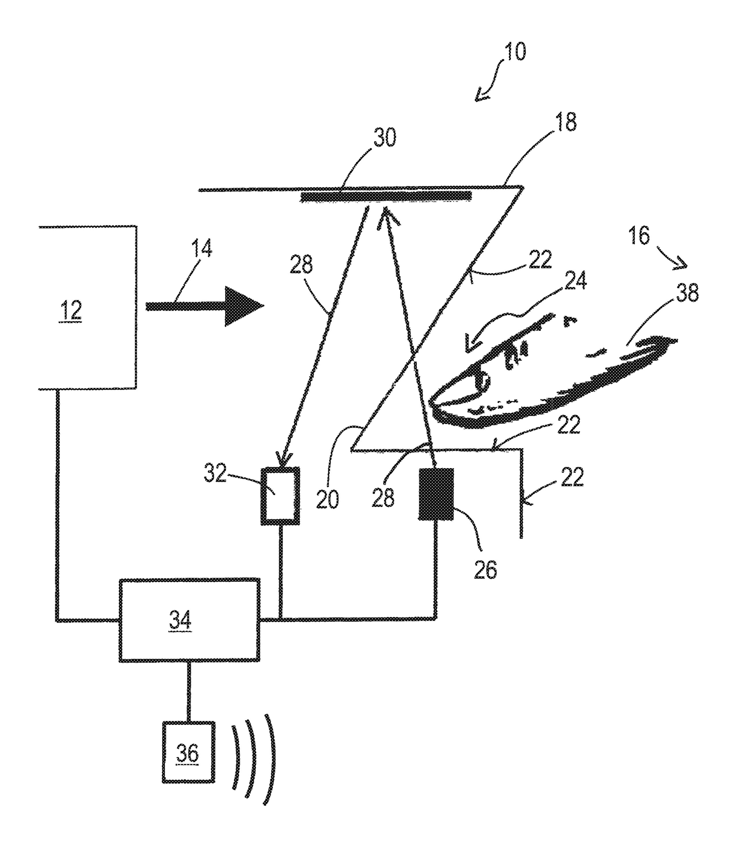
The present invention relates to an optoelectronic sensor for monitoring a monitored zone, having a main light transmitter for transmitting sensing light signals that propagate through a protective screen into the monitored zone; having a main light receiver for receiving light that emanates from the monitored zone; and having a control unit for
