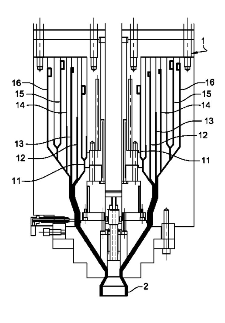
a second material distinct from the first material, such that during the second period of time the coextrusion head produces a second multilayer parison from which the diesel tank or filler pipe can be manufactured.
