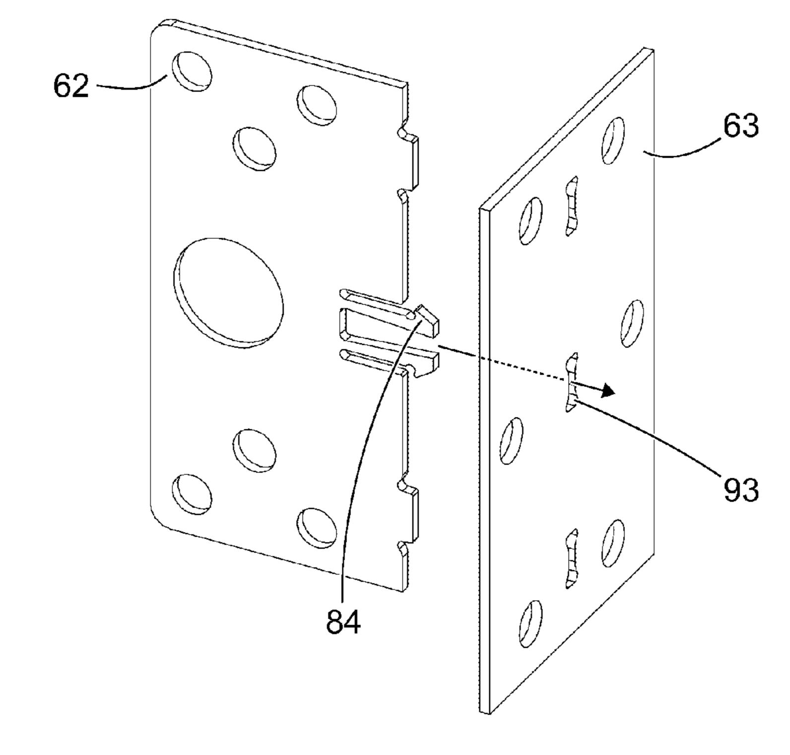
Fig. 20 62 61 63 63 62 61 64 62 61 63 62 Fig. 21 \_101 cutting out flat structures \_102 bending one of the flat structures \_103 joining the flat structures to form a strut joining the ends of the strut to node structures \_105 joining the node structures and further struts
