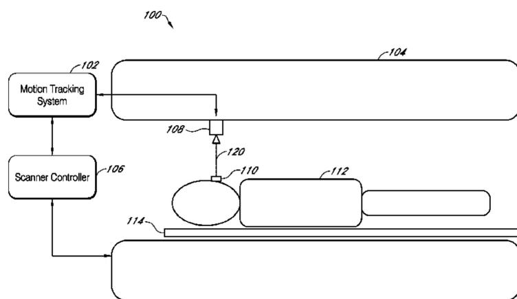
the tracking information to a scanner controller to enable compensation within a medical imaging scanner for object motion.
