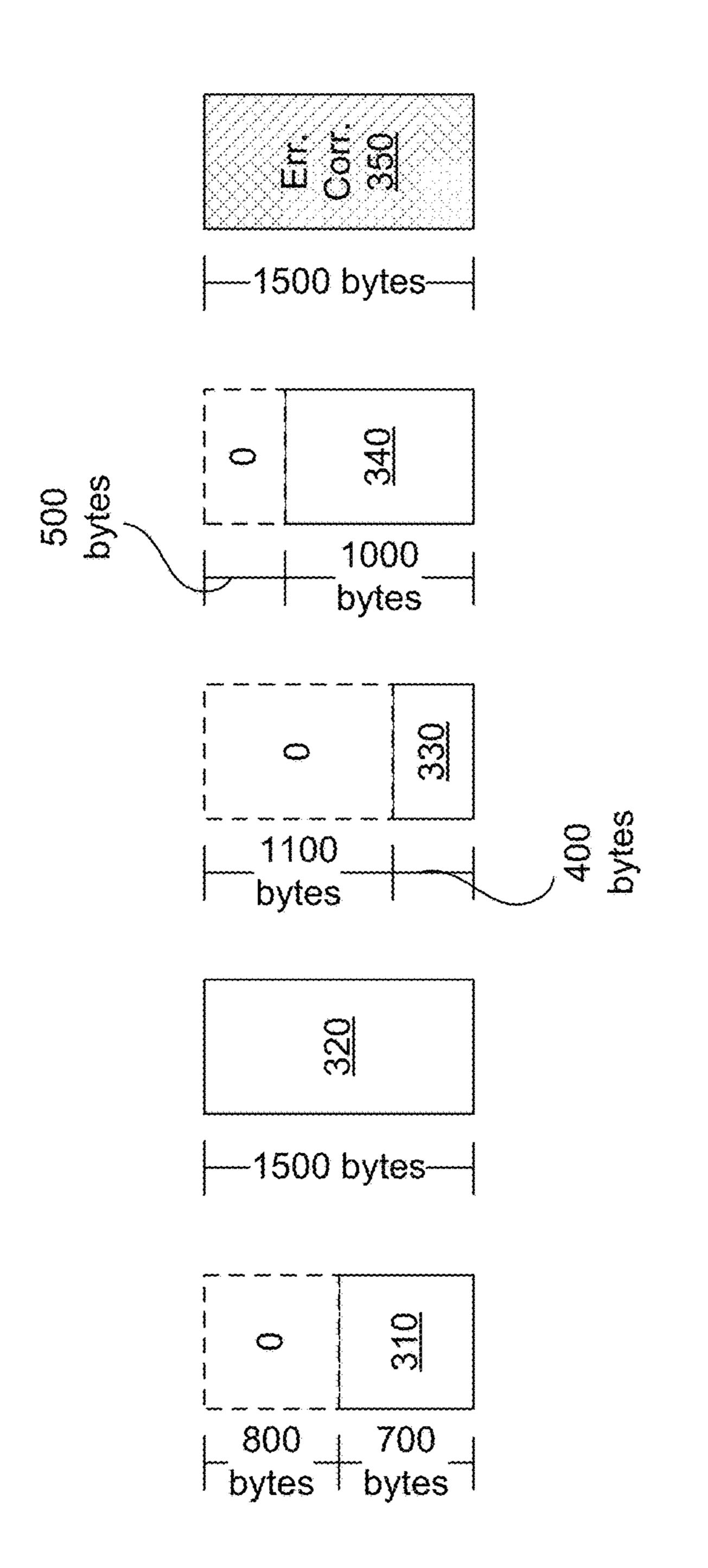
ATA: 700 + 1500 + 400 + 1000 = 3600 bytes CORR: 1500 bytes Corr. Packet Ratio = 1:4 (20% overhead)
