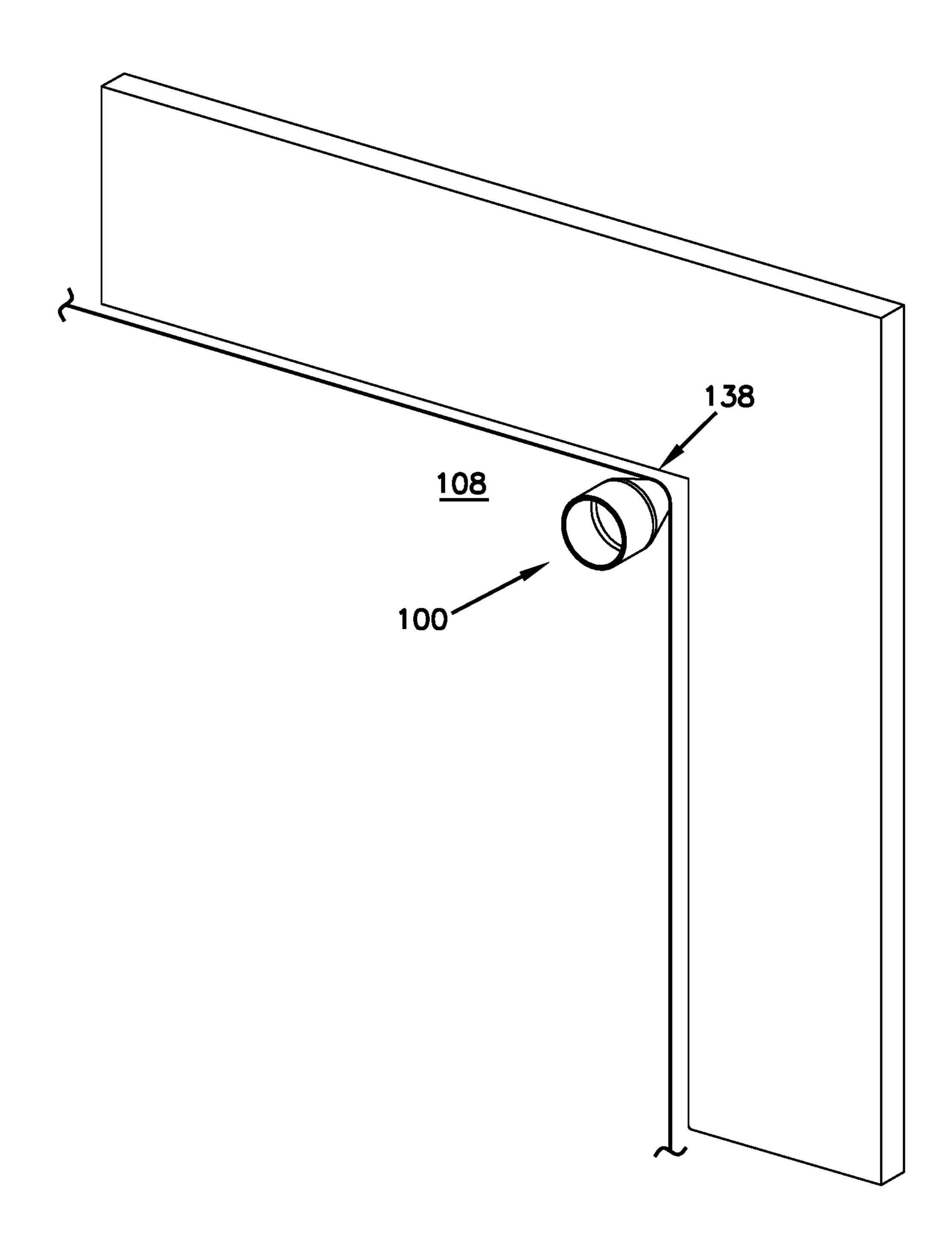
200 FIG. 7 202 ENGAGE HOLDING TOOL WITH CABLE GUIDE DEVICE 204 HOLD CABLE GUIDE DEVICE AT WORK AREA 206、 ROUTE CABLE AROUND CABLE GUIDE DEVICE 208, FIX CABLE TO WORK AREA 210, REMOVE CABLE GUIDE **DEVICE**
