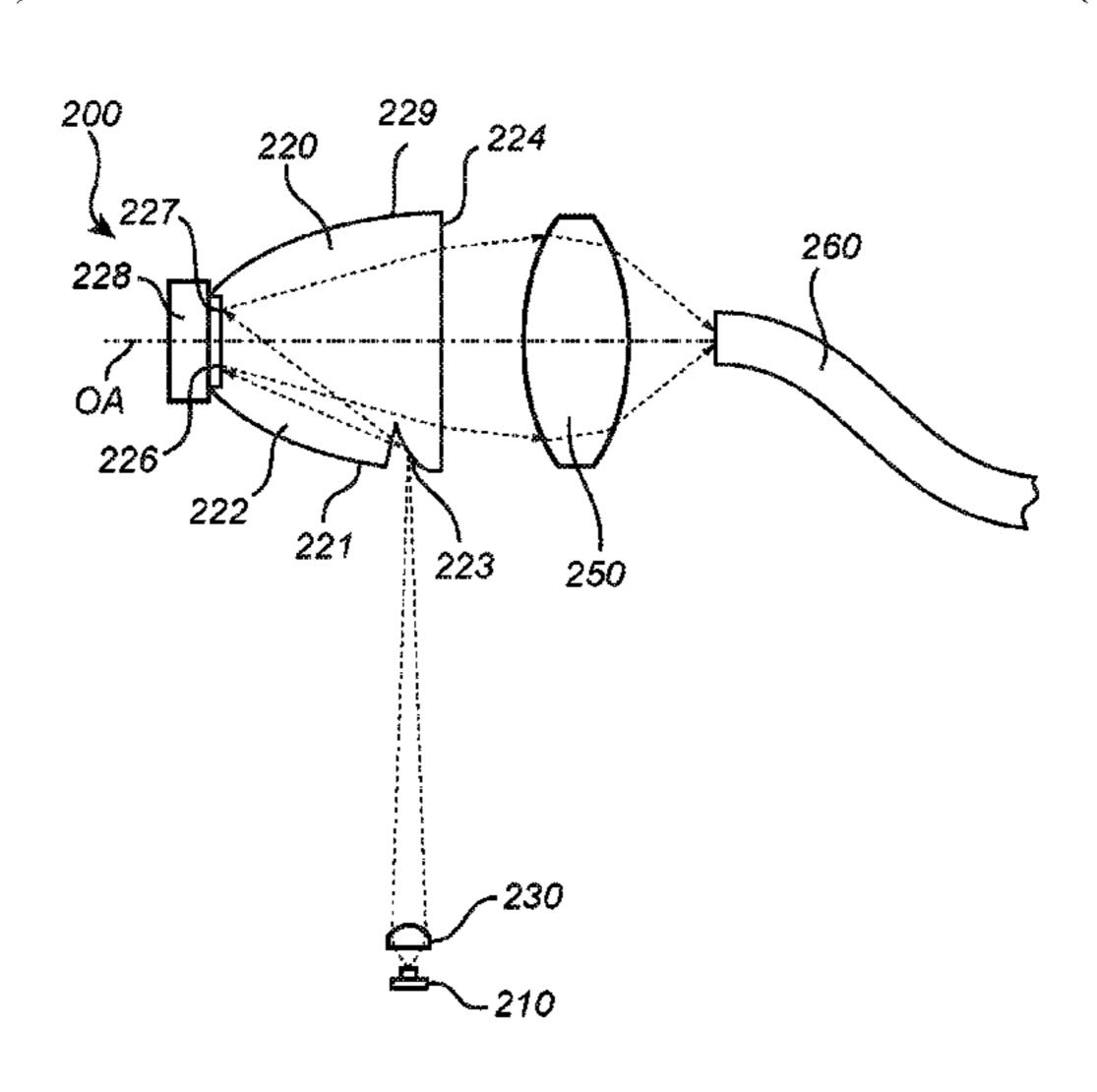
the light entrance is arranged at a geometrical envelope surface surrounding the main optical axis of the light guide.
